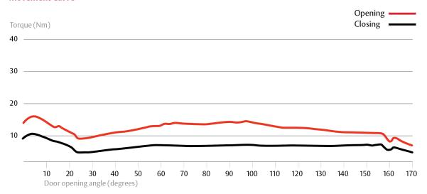
**Note:** Movement curve represents approximate forces required to operate a size 1 door closer. The illustration is an approximation based on one set of parameters. Any change to these parameters will result in a variation of performance.
