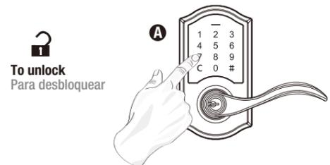
Enter the correct user code or programming code. Upon the green indicator light on and a short beep heard, turn the outside lever to unlock.
