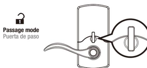
Rotate the interior thumbturn from horizontal to vertical position as shown to set your lock to passage mode. The lockset is then served as a passage lever.
