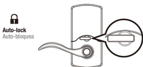
Turn the interior thumbturn from vertical to horizontal position to enable auto-lock mode.
