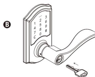
Use a mechanical key to lock or unlock.
