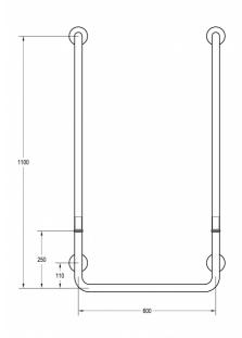
$<sup>^{\</sup>star}$  Compliant with the Force Requirements within AS1428.1: 2021, Section 14.
