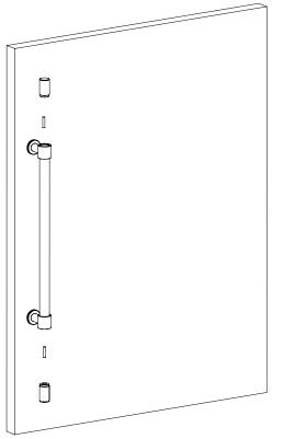
Once secured, install bar end pieces and tighten
