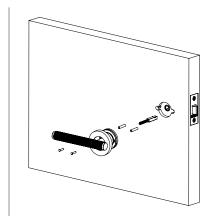
Repeat above step hand tightening M4x30 screws
